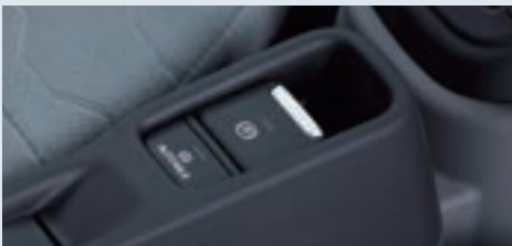
• Electric parking brake panel
