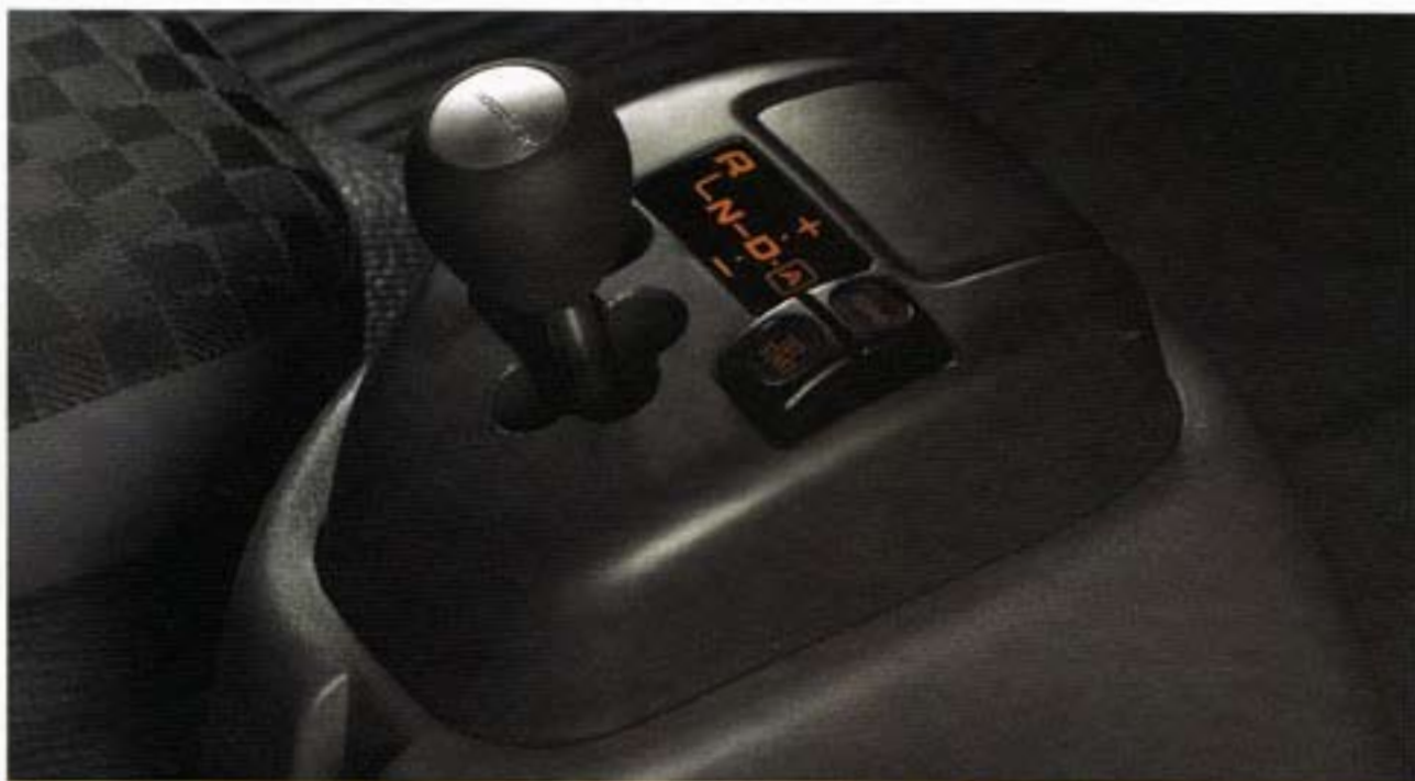
Gear selection: move the selector to the right to engage automatic and forward or back to change ratio in the five-speed gearbox
