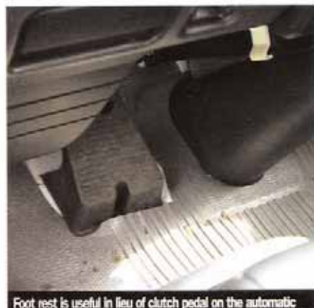
Foot rest is useful in lieu of clutch pedal on the automatic
